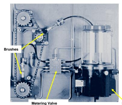
Brush type chain lubrication systems can provide a simple, inexpensive, reliable, maintenance friendly way of applying chain oils and lubricants.
